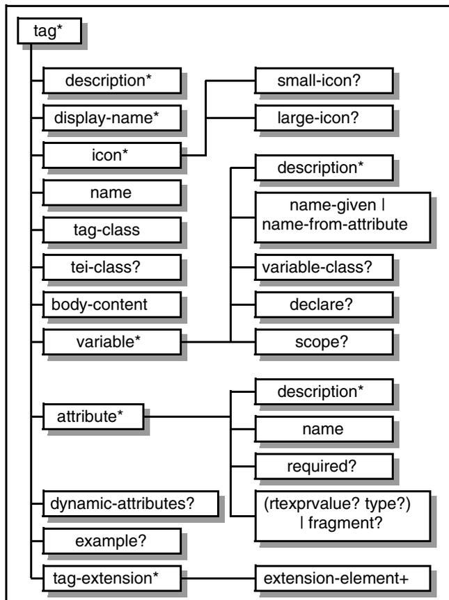
**Figure JSP.C-8** TLD Schema Element Structure - tag
