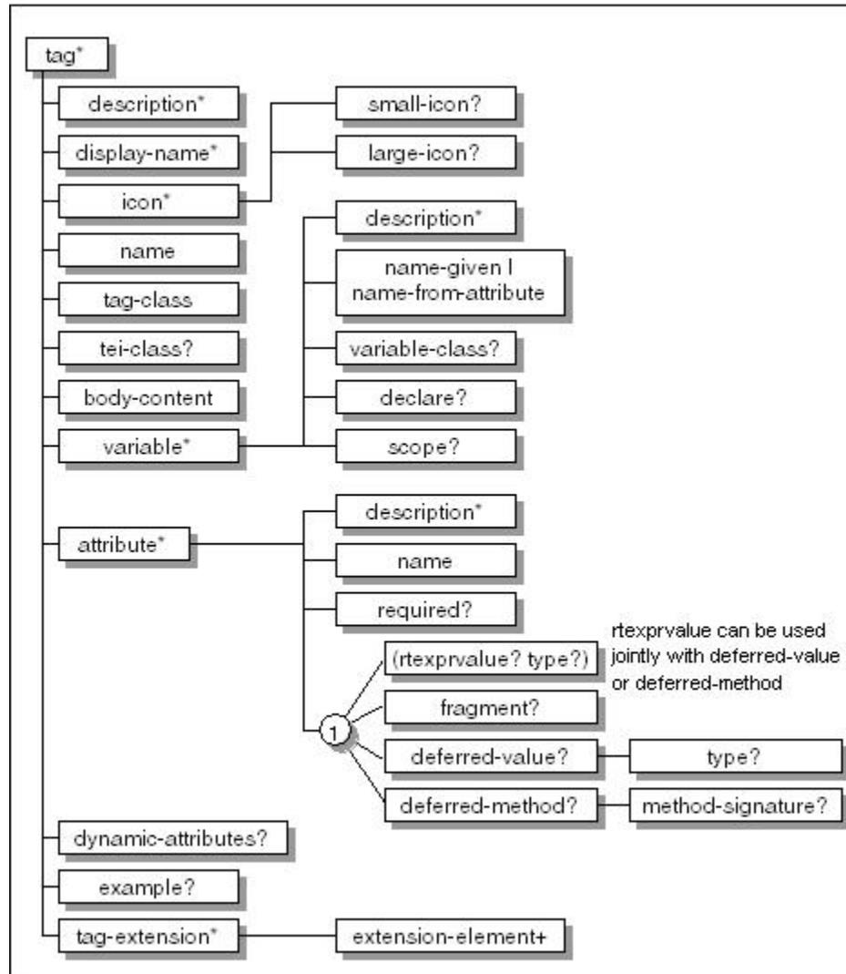
**Figure JSP.C-3** TLD Schema Element Structure - tag
