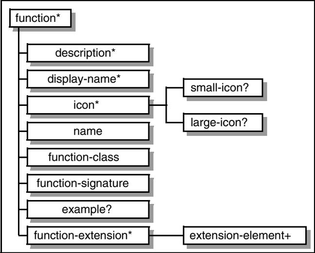
Figure JSP.C-10 TLD Schema Element Structure - function
