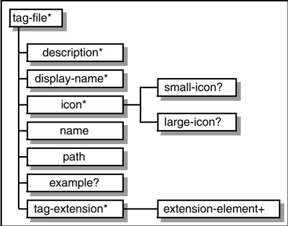
Figure JSP.C-9 TLD Schema Element Structure - tag-file
