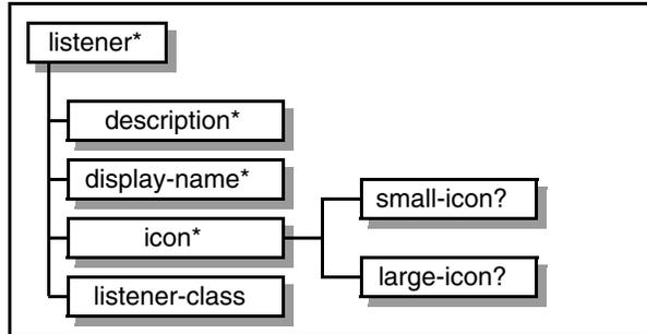
**Figure JSP.C-7** TLD Schema Element Structure - listener
